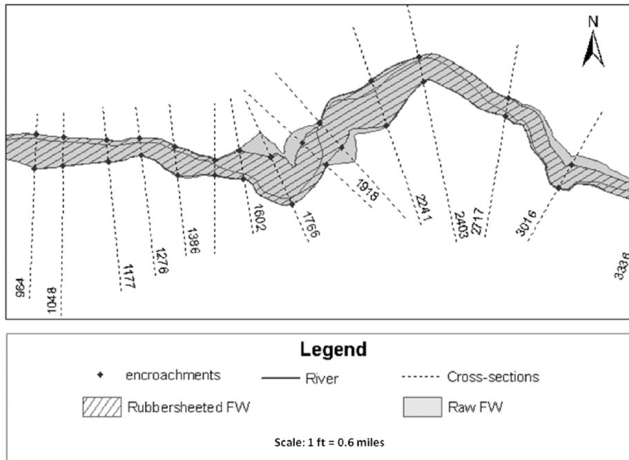
Figure 9: Comparison of the raw floodway and rubbersheeted floodway
