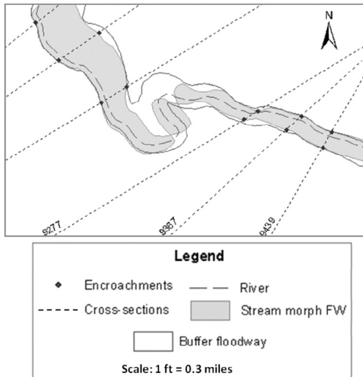
Figure 6: Map showing buffer floodway method vs. Stream morphing method
