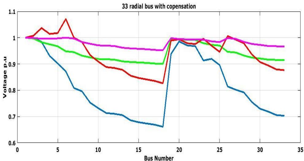
**Figure 1: 33 Radial bus with voltage stability compensation**
