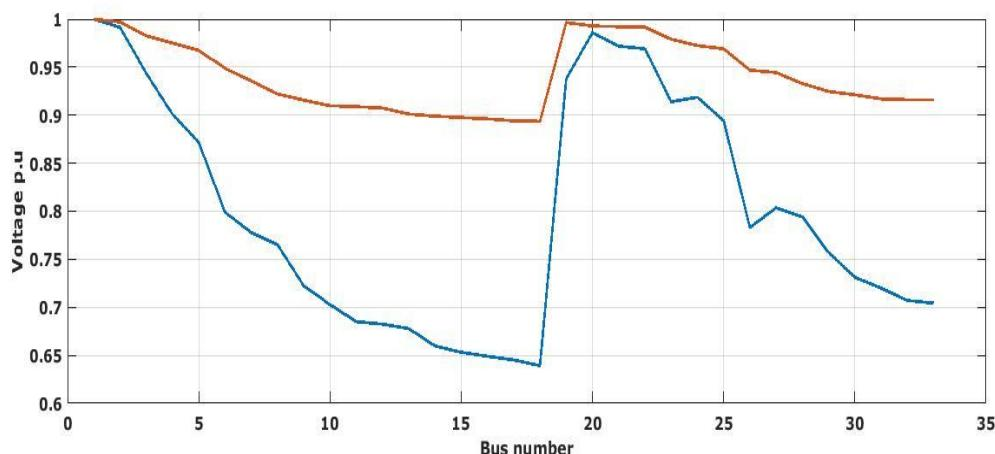
**Figure 2: 33 Radial bus with voltage stability compensation**
