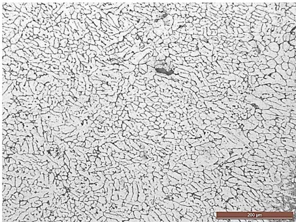
Fig.4. Micro-structure of specimens prepared in the absence of vibrations (200X)
