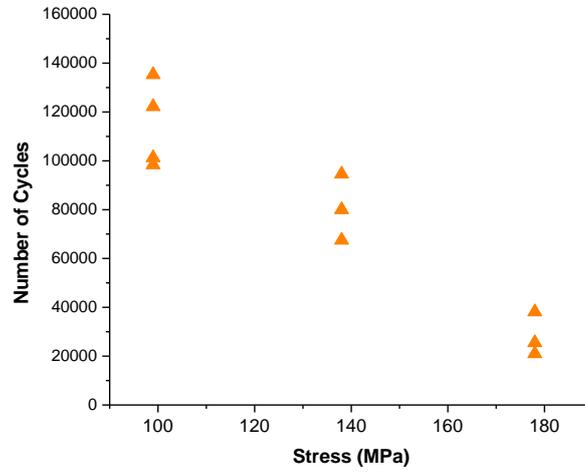
Fig.1. Number of Cycles vs. Stress (Without vibrations)
