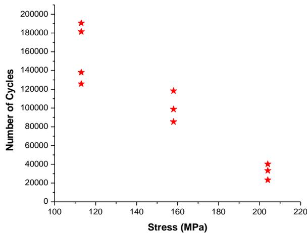
Fig.2. Number of Cycles vs. Stress (at 160V vibrations)
