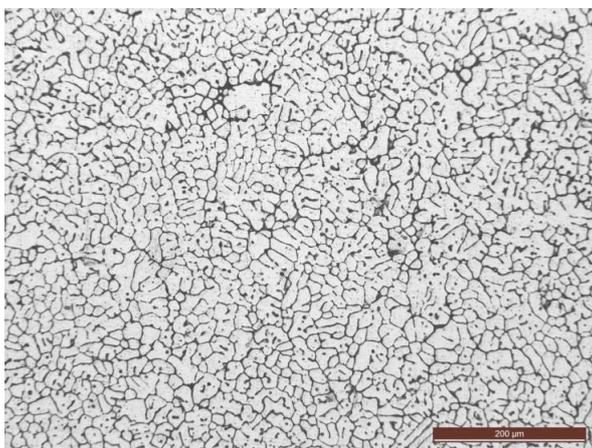
Fig.5. Microstructure of specimens prepared at with 160V vibration condition (200X )
