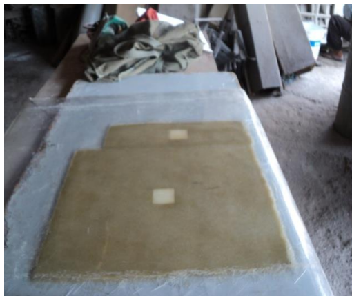
Figure 5.7: Keep the Specimens for Curing and Cut Them as Per the Required Dimensions
