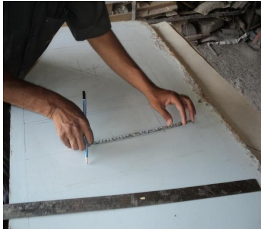
Figure 5.2: Preparing the Mould for Specimens.
