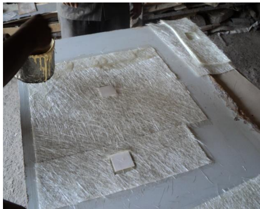
Figure 5.6: Applying the Alternate Layer of Resin and Glass Fiber Sheet.
