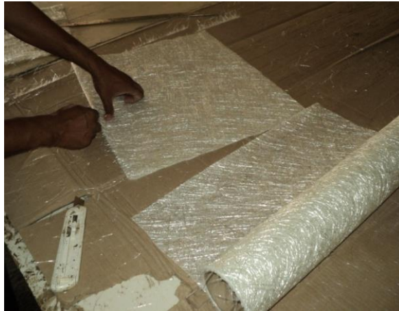
Figure 5.5: Cutting the Glass Fiber Sheet as Per Requirement
