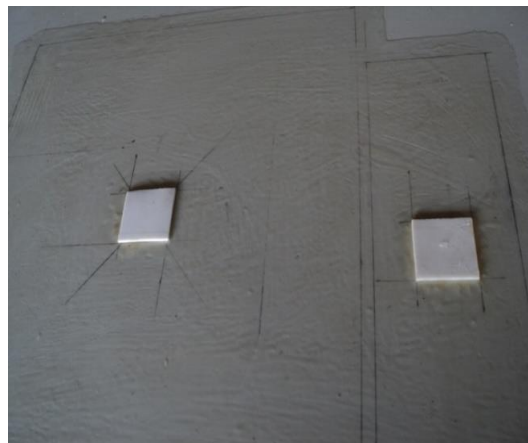
Figure 5.4: Prepare the First Layer of Resin and Placing the Teflon Slice on It
