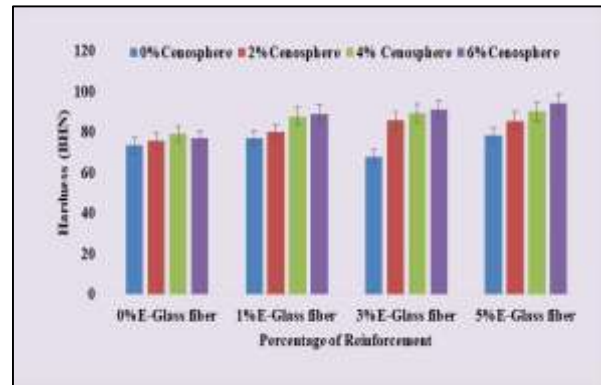
Fig.5d. Difference in hardness with dual reinforcements (8Hour aged)
