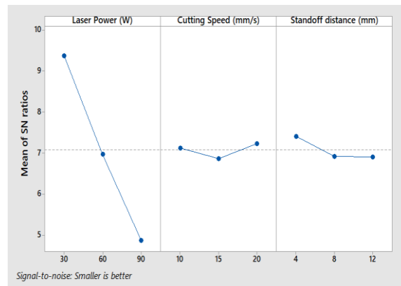
Figure 7: Main effect plot for kerf width
