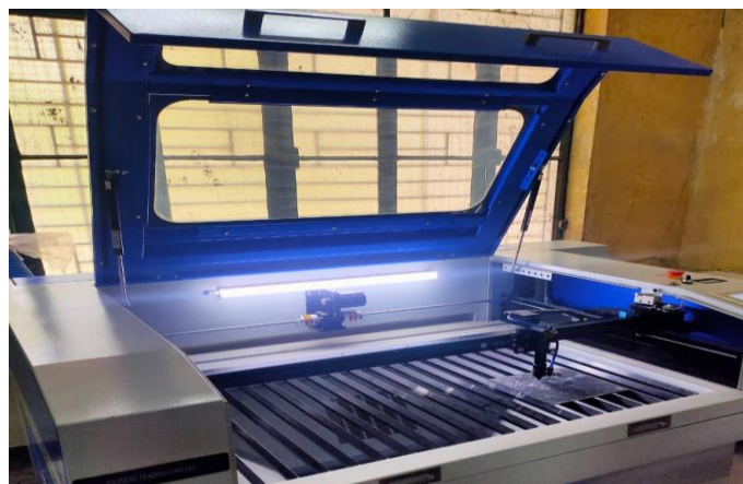
Figure 6. CO 2 laser cutting of hybrid natural fibre coir-carbon epoxy composites
