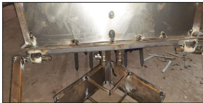
Fig 8. Fertilizer dispenser at the bottom
