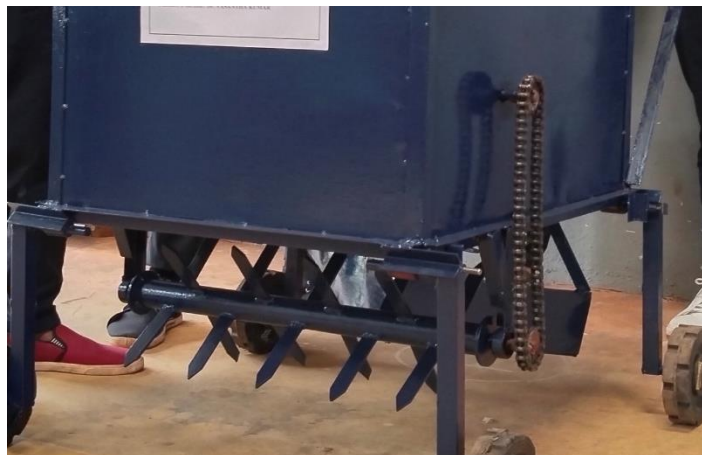
Fig 9. Chain sprocket & rotating blades
