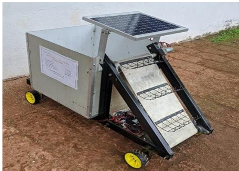
Fig. (9): Isometric view of fabricated Hybrid Cleaning Rover
