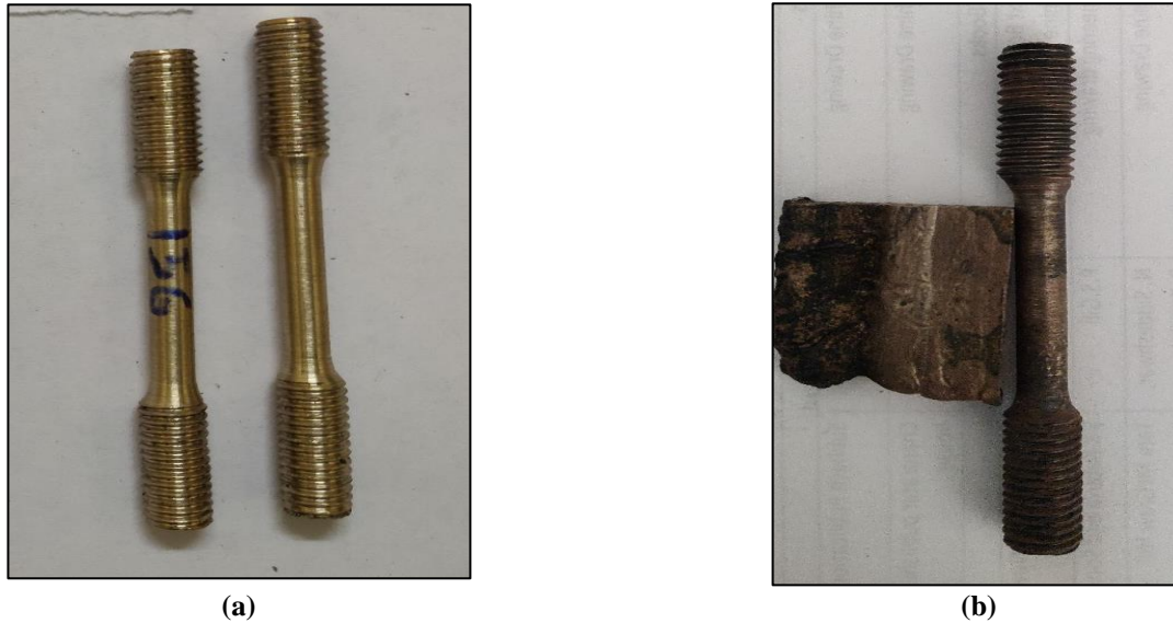
Fig. 2: Photographs of Alloy 1 in (a) cast and (b) heat treated conditions Sample composition and their respective designations
