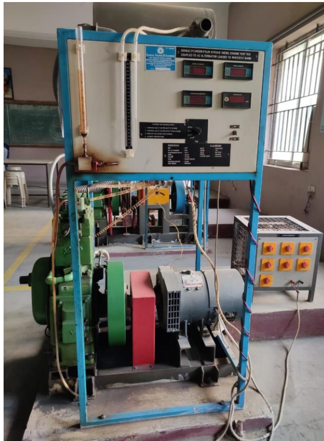
Fig. 1. Engine Setup is a single-cylinder CRDi Kirloskar
