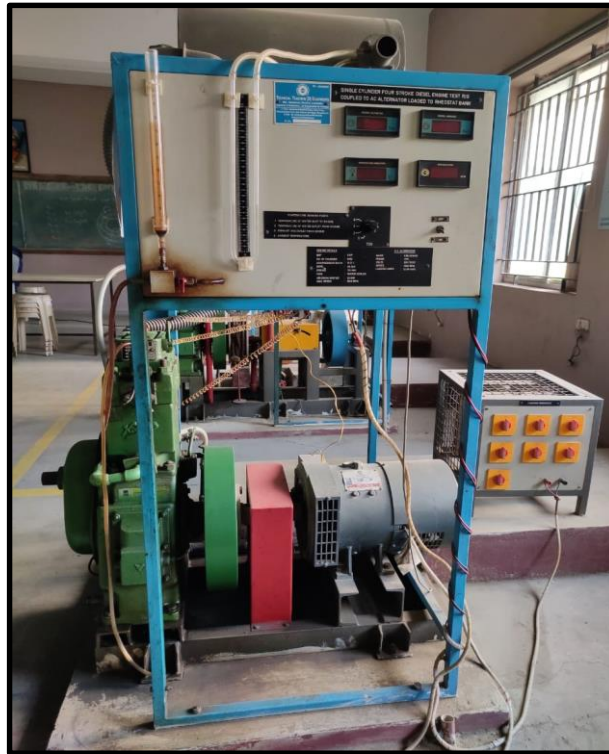
Fig. 1. Engine setup is a single-cylinder Kirloskar bore, stroke length mounted on the same base frame with eddy current.
