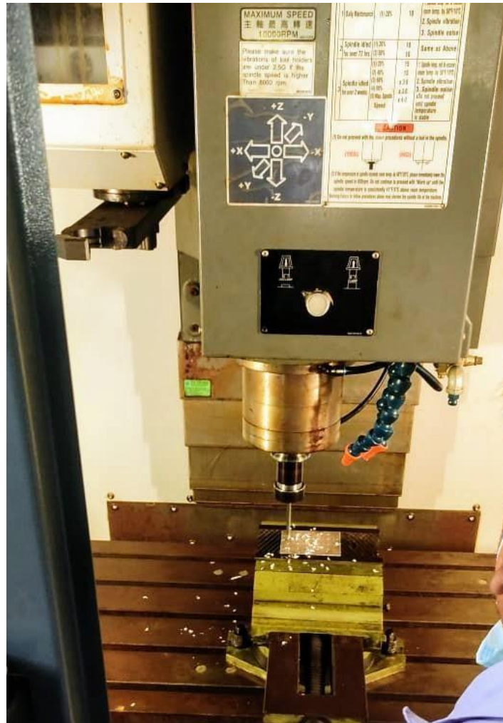
Fig. 1. Drilling machine - drilling capacity - \varnothing 25 mm. Table size - 400 mm, range of speed 2000- rpm, feed rate-0.5 -1.5 mm/min, depth of cut - 0.3 to 0.7, tool diameter- 10 mm .
