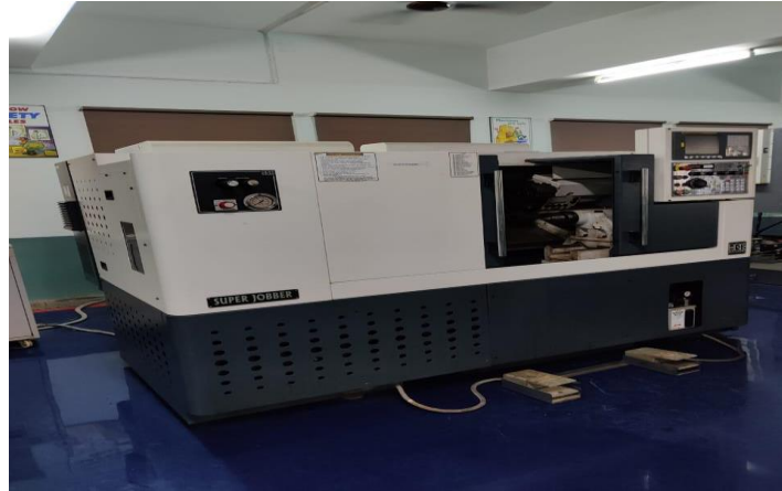
Fig. 3. CNC Turning Machine-ACE. The specifications of CNC turning machine are: Dia of turning (Max) - 320 mm, Length of turning (Max) - 400 mm, Centre distance - 425 mm, Speed of spindle (Max) - 3500 rpm, Stations - 8, Bed swing -500 mm, Carriage swing - 260 mm. The input variables speed of cut, rate of feed and depth cut were set as 175 m/min, 0.150 mm/min and 0.6 mm respectively.
