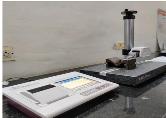
Fig. 4. Surface roughness tester - Surftest SJ - 410 - Range of measuring X-axis - 25 mm (1inch); Z1-axis - 800 \mu\text{m} , 80 \mu\text{m} , 8 \mu\text{m} ; Measured speed - 0.05 \mu\text{m}/\text{sec} ; Measuring force - 0.75 mN; parameters - Ra, Rz, Rt, Rp, Rv; Measured profiles - roughness; graph analysis - BAC and ADC curves; cutoff length - 0.25 mm.
