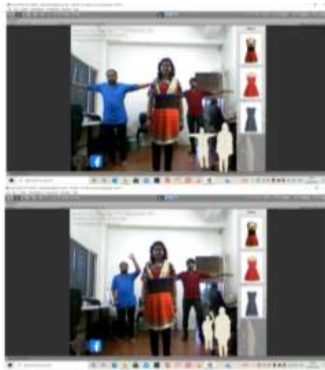
Fig No. 10 illustrates demonstration of Multiple User Detection Testing Module. In this module one user is continue to use system and multiple user comes in background. Kinect can detect multiple user but it will work for the first user detected with calibration pose.
