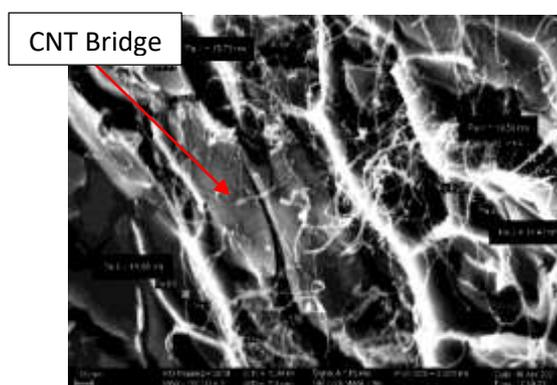
Fig.9. CNT bridge in 1.25% sample
