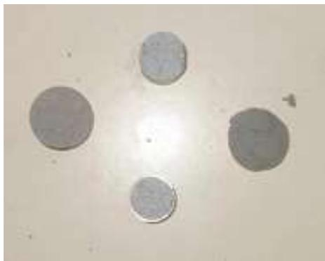
Fig.7: Specimen prepared for Fe-SEM test.
