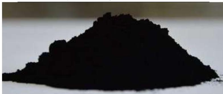
Fig.2: Multiwalled carbon nanotube powder
