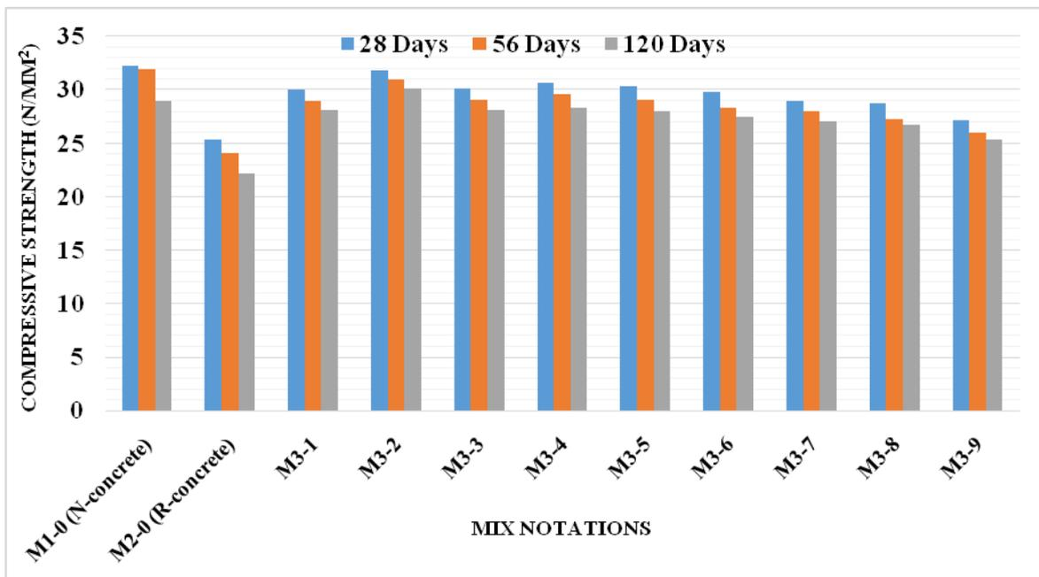
Fig. 2 Compressive strength of concrete specimens after immersion in 4.0% MgSO<sub>4</sub>
