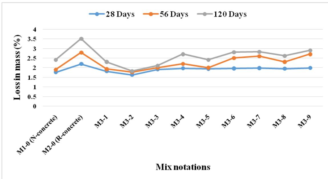
Fig. 4 Loss in mass due to sulphate attack
