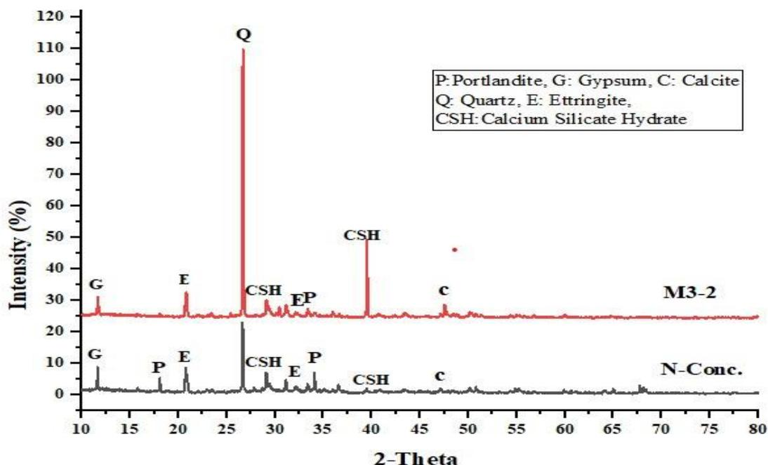
Fig. 5, XRD patterns of specimens after 120 days of magnesium sulphate exposure
