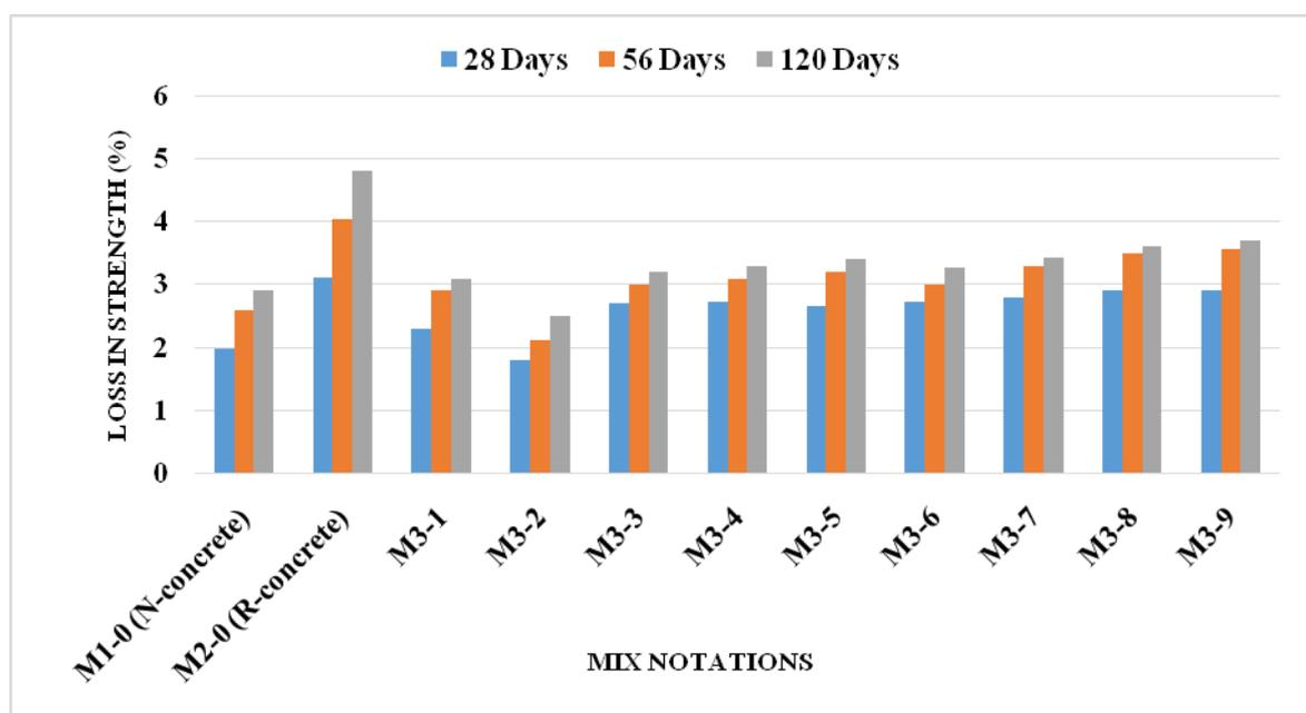
Fig. 3 Loss in strength due to MgSO<sub>4</sub> exposure.
