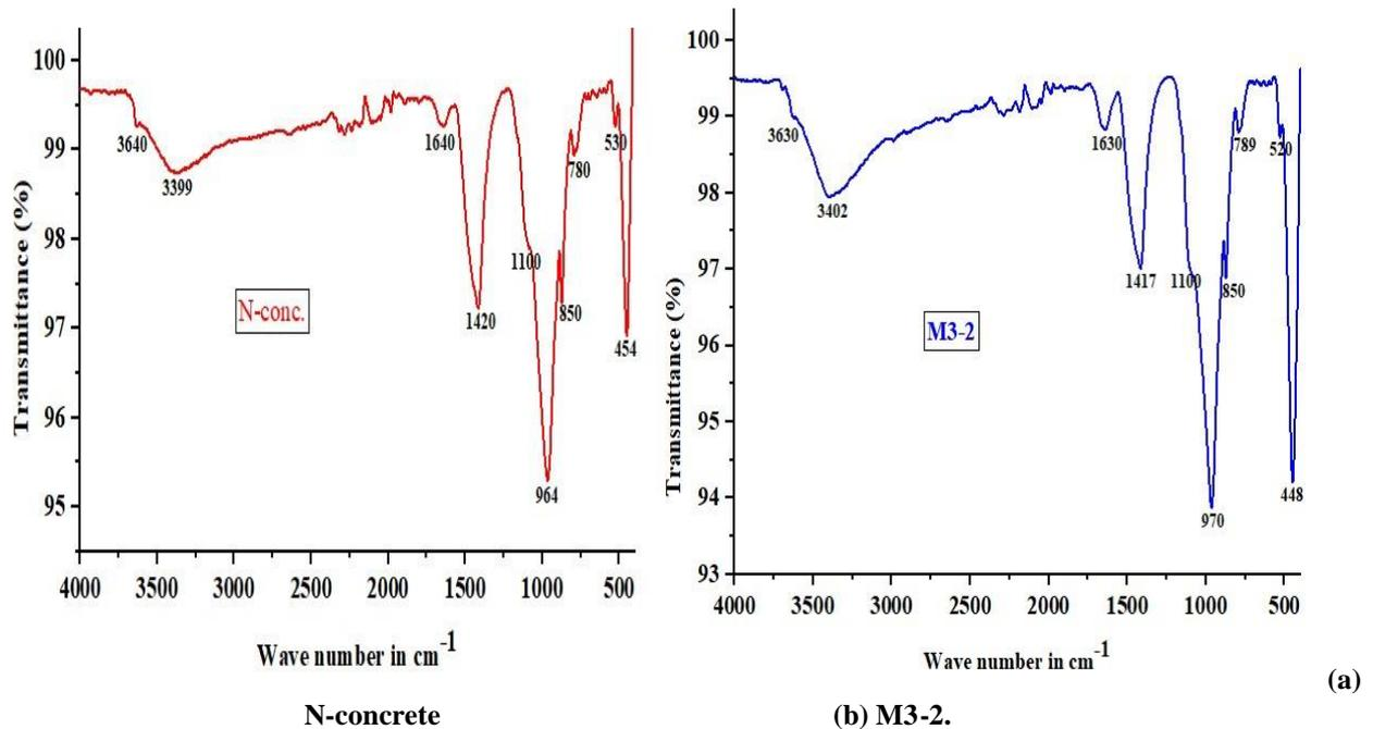
**Fig. 5, FTIR spectra of specimens after 120 days of magnesium sulphate exposure**
