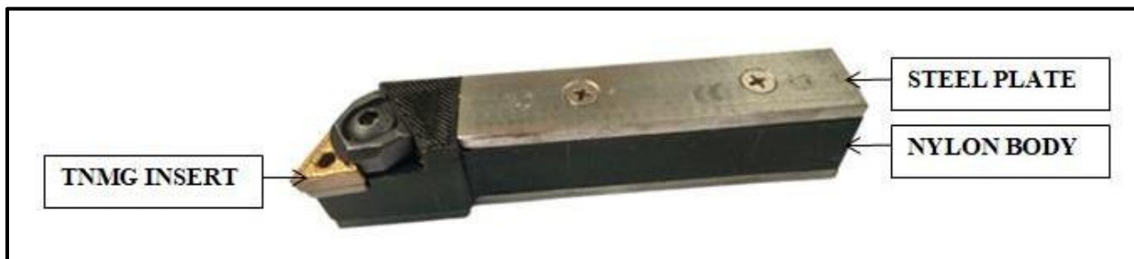
Fig. 1 FFF 3D Printed Flitched Tool holder for TNMG Insert
