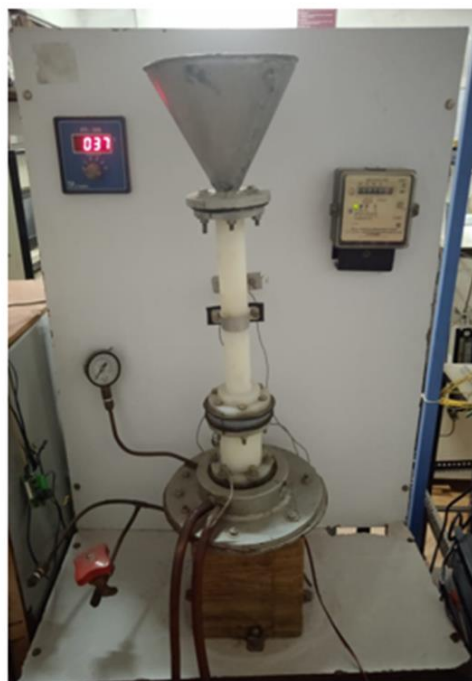
Figure 1: Experimental Setup of Thermoacoustic Refrigerator
