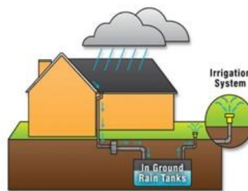
Fig. 5 Rain Water Harvesting System
