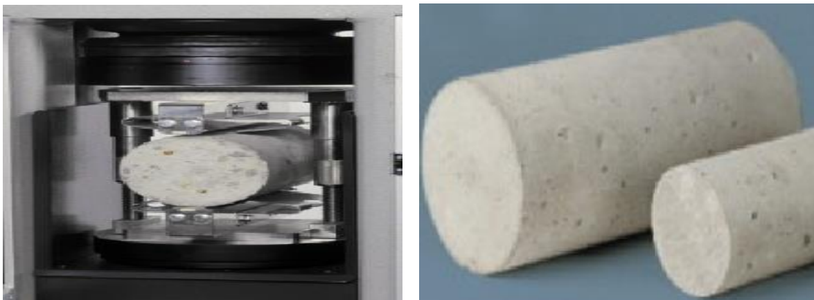
Fig. 4. Cylinder concrete test specimen and split tensile test.
