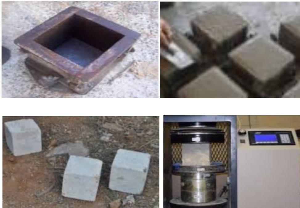
Fig. 3. Cubic test samples and compressive test.
