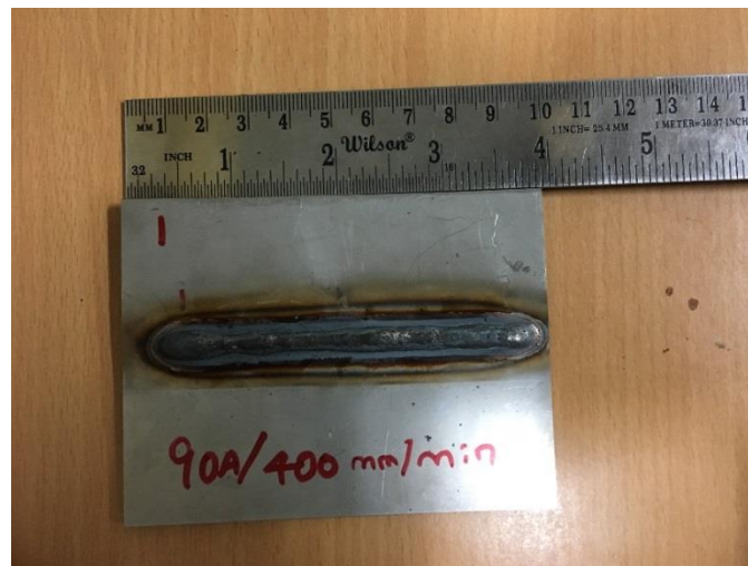
Figure 13 Welded sample of 316L using CMT
