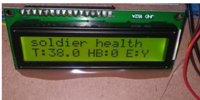
Figure 7: Parameters displayed on LCD (Emergency)
