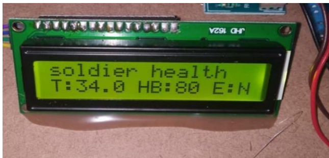
Figure 6: Parameters displayed on LCD (No emergency)
