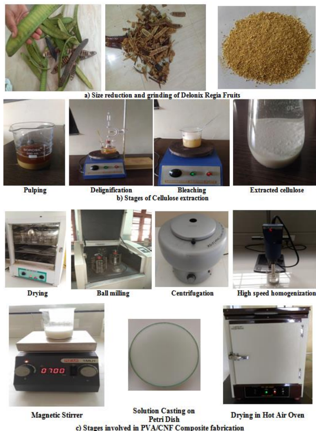
Fig. 1: Procedure for preparation of PVA/CNF Composite
