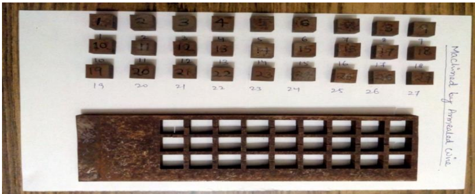
FIG. 3: MACHINED WORK PIECES OF D2 STEEL BY USING ANNEALED COPPER WIRE
