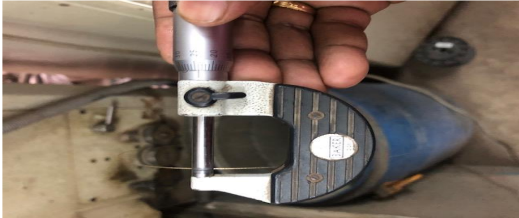
FIG. 5: SCREW GAUGE WHILE MEASURING WIRE DIAMETER
