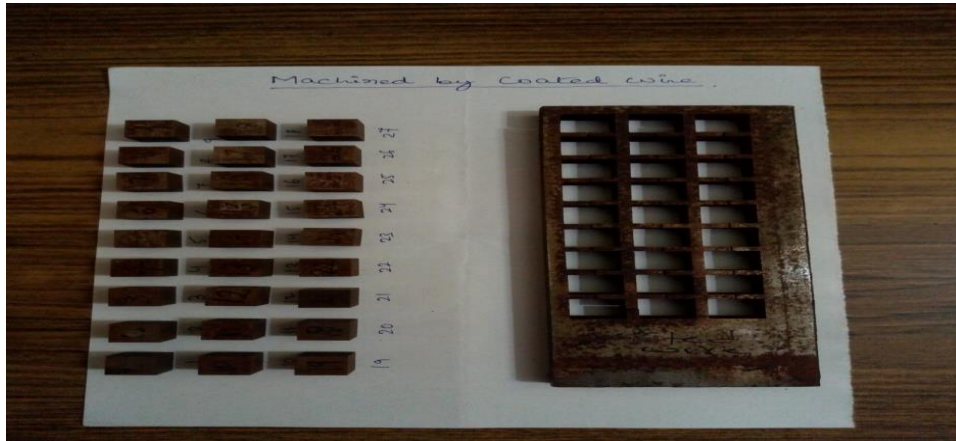
FIG. 2: MACHINED WORK PIECES OF D2 STEEL BY USING COATED COPPER WIRE
