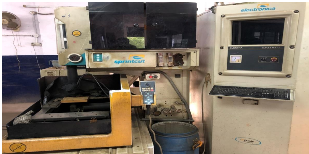
FIG. 1: ELECTRONICA SPRINT CUT WIRE EDM MACHINE
