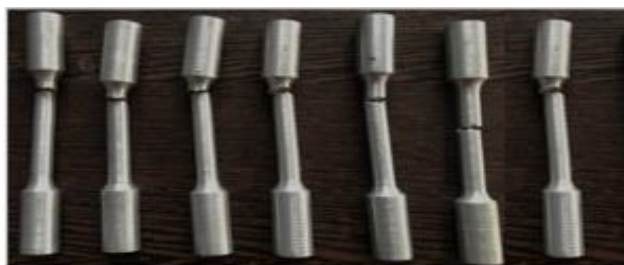
FIGURE 3. Tensile fractured specimens
