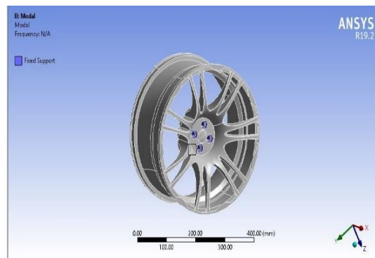
Fig: 6.1 Wheel studs fixed at center plain axis
