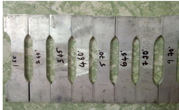
Fig 2: Tensile test samples
