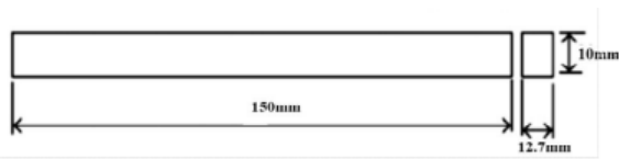
Fig 5: Schematic diagram of Flexural test specimen
