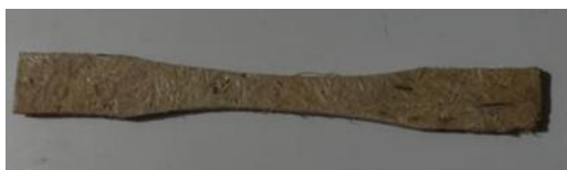
Fig 4: Dog-bone specimen of the composite
