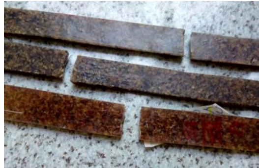
Fig.5 Failed specimens during tensile test
