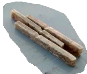
Fig. 6 prepared impact samples
