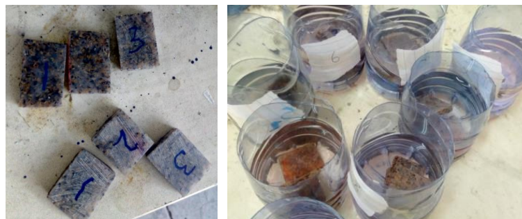
Fig. 7 water absorption test samples and water absorption test respectively
