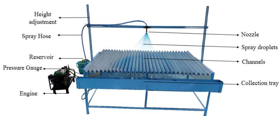
FIGURE 1. SPRAY PATTERNATOR
