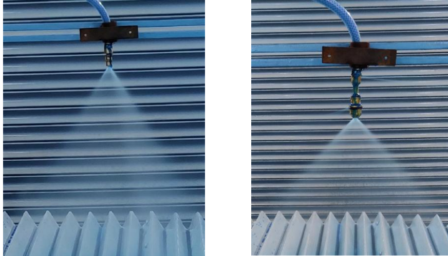
FIGURE 3 SPRAY DISTRIBUTION - NMD AND NTM NOZZLE
