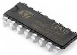
L293D is a dual H-Bridge motor driver, so with one IC we can interface two DC motors which can be controlled in both clockwise and counter clockwise direction and if you have motor with fix direction of motion the you can make use of all the four I/Os to connect up to four DC motors. L293D has output current of 600mA and peak output current of 1.2A per channel. Moreover for protection of circuit from back EMF
