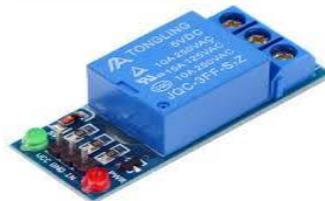
Relays are used in a wide variety of applications. The advantage of relays is that it takes a relatively small amount of power to operate. Relays are simple switches which are operated both electrically and mechanically. Relays consist of an electromagnet. It also contains a set of contacts. The switching mechanism is based on electromagnet. Most of the devices have the application of relays.
