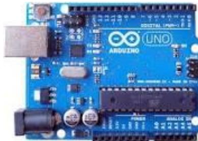
The **Arduino Uno R3** is a microcontroller board based on the ATmega328 (datasheet). It has 14 digital input/output pins (of which 6 can be used as PWM outputs), 6 analog inputs, a 16 MHz crystal oscillator, a USB connection, a power jack, an ICSP header, and a reset button. It contains everything needed to support the microcontroller; simply connect it to a computer with a USB cable or power it with a AC-to-DC adapter or battery to get started.
