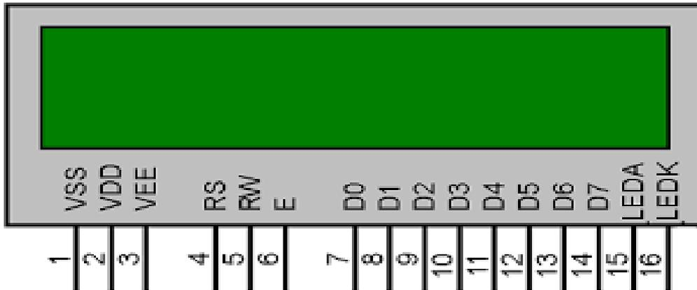
It is called Liquid Crystal Display. We are going to use 16x2 characters LCD. This will be connected to microcontroller. The job of LCD will be to display all the system generated messages coming from the controller. LCD will provide interactive user interface. This unit requires +5VDC for its proper operation. This module is used for displaying the present status of the system.
