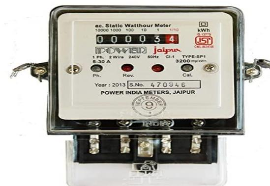
Energy meter or watt-hour meter is an electrical instrument that measures the amount of electrical energy used by the consumers. Utilities is one of the electrical departments, which install these instruments at every place like homes, industries, organizations, commercial buildings to charge for
