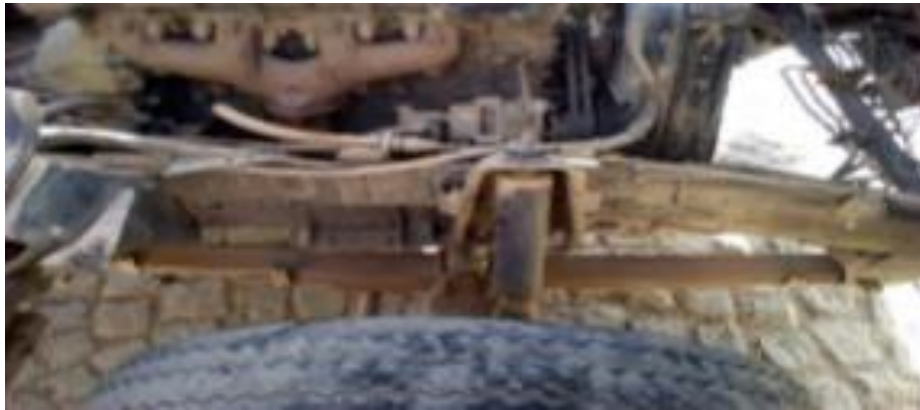
Figure 4: Mounting of steel leaf spring [Observation]
