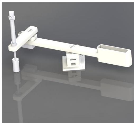
**Fig.1** Scara Manipulator
