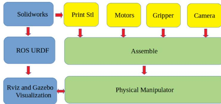
**Fig.2** Schematic of Design
