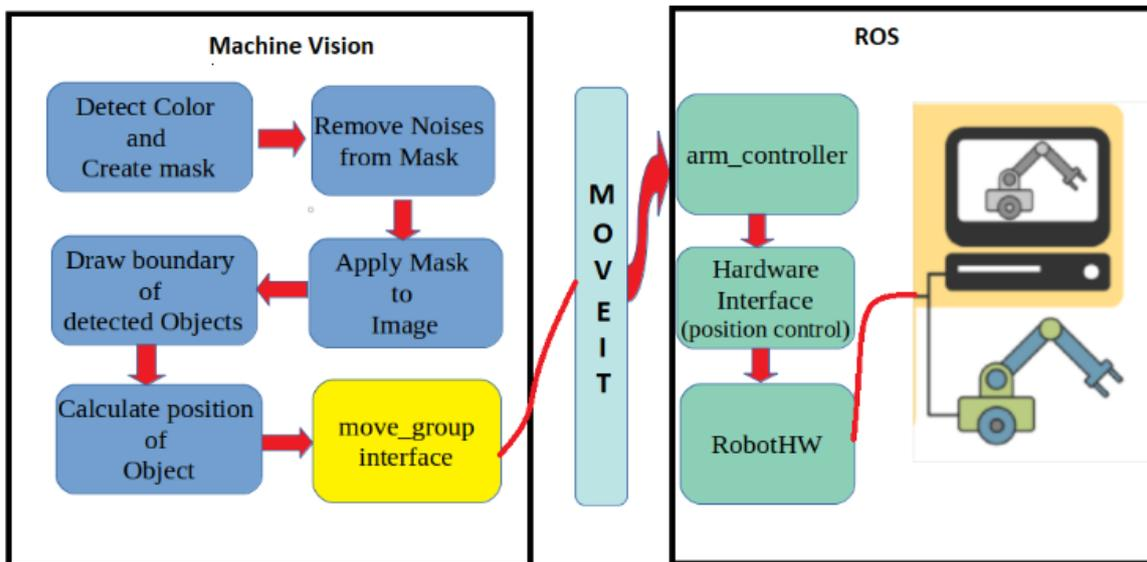
**Fig.7** Schematic of Machine Vision and Entire Process
