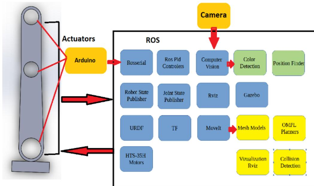
**Fig.5** Real Manipulator and and Software in Ros Frame.
