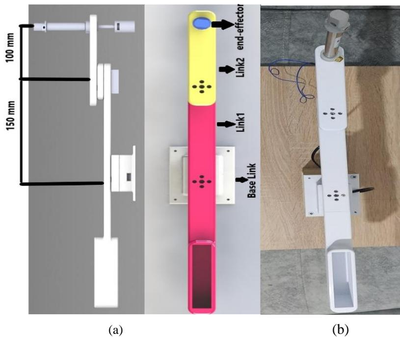
**Fig 4.** a) Solidworks Design b) Assembled Manipulator
