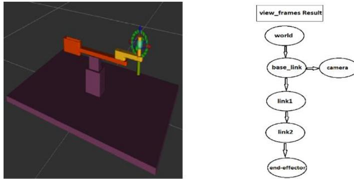
**Fig.6** a)Manipulator Displayed in Rviz b) Ros view\_frames and rqt\_tf\_tree Results
