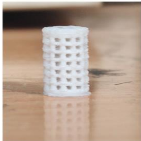
Fig. 4. 3D printed PLA specimen (Experiment no 27)
