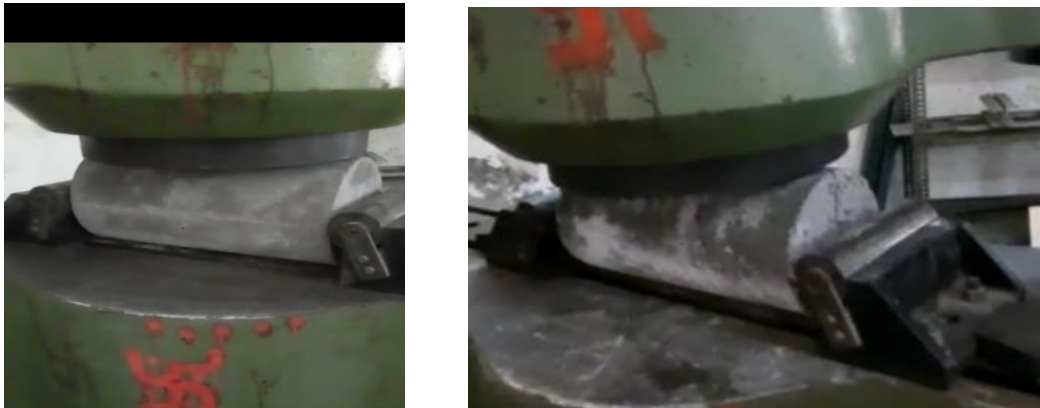
Figure 2: Cylinder Cracked during split tensile strength test
