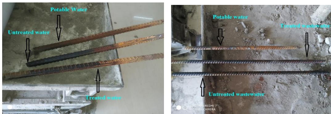
Figure 17: Effect of corrosion on reinforced bars
