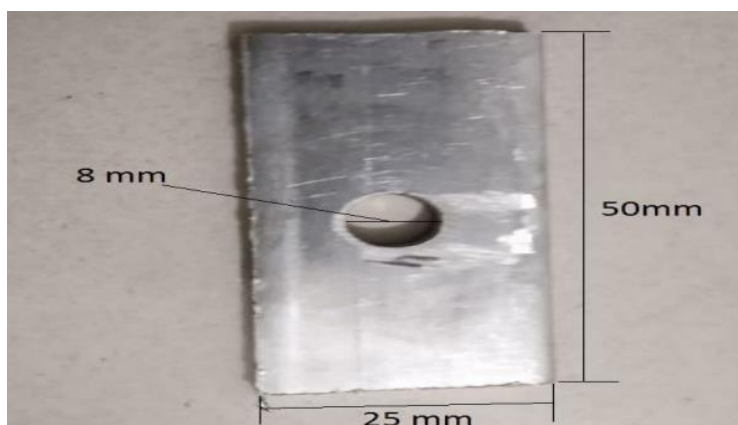
Figure 1: Prepared Specimen of SS 430
