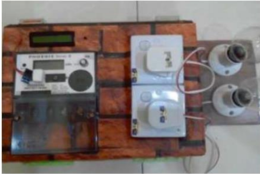
Figure 2: Energy meter with loads of 2 lamps
