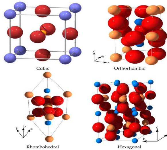
**Fig-1 Structure of perovskite material**
