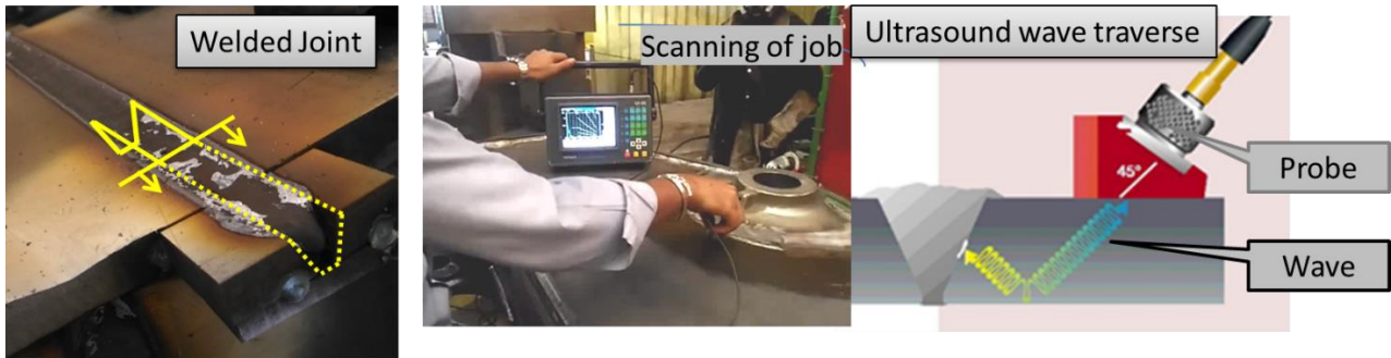
Fig. 1. Details of the ultrasonic testing process explained
