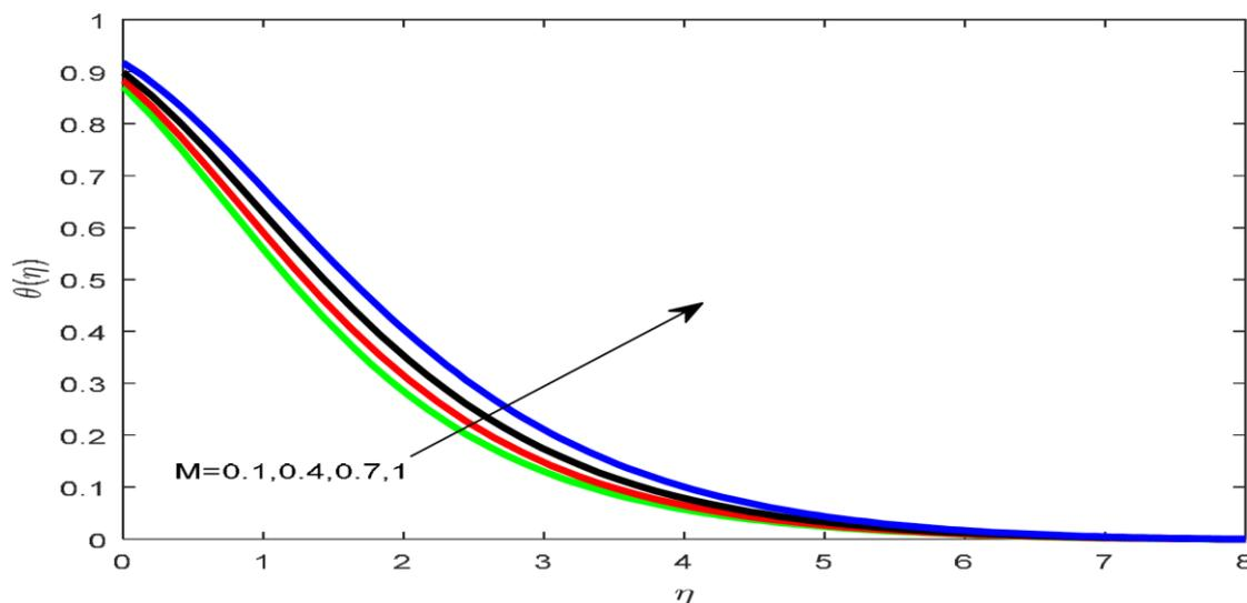
Image.3 Impact pertaining to M based upon thermal field.
