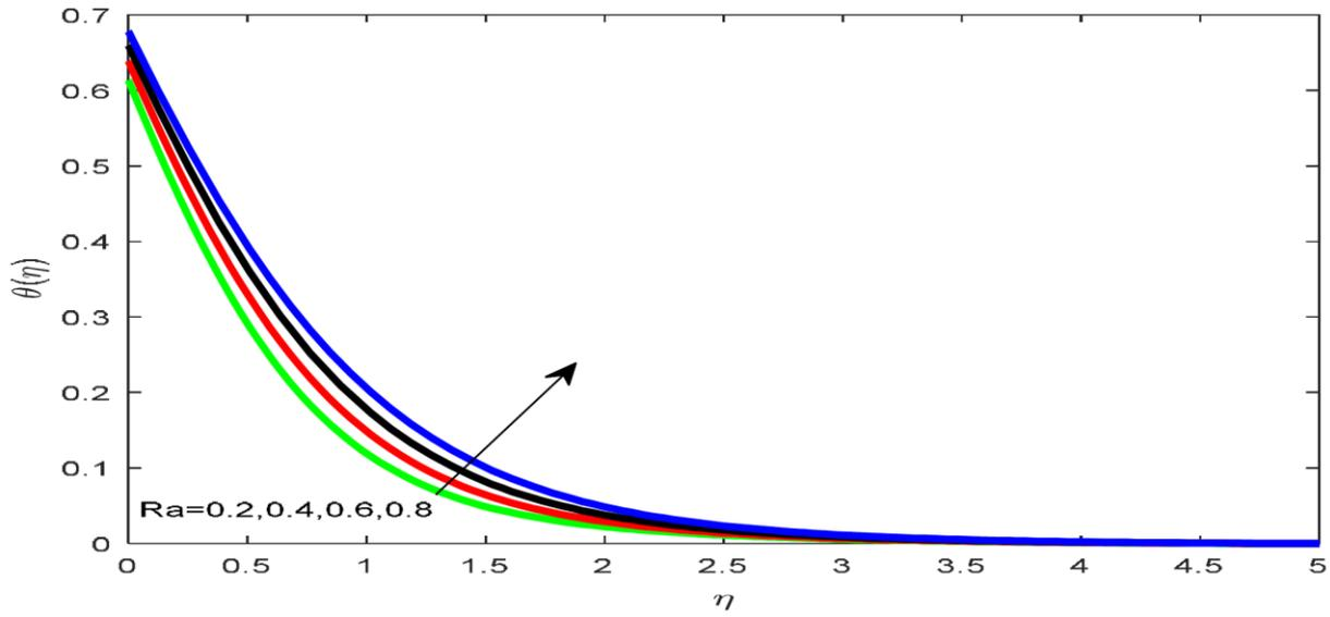
Image.6 Impact pertaining to  $Ra$  based upon thermal field.
