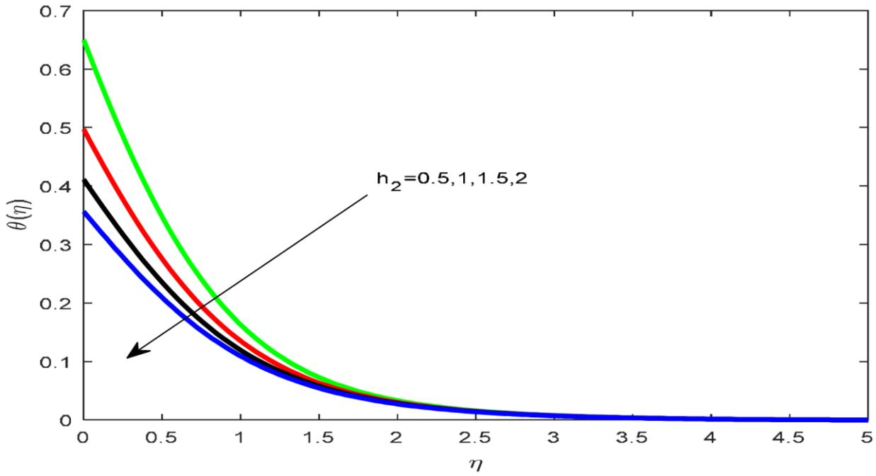
Image.12 Impact pertaining to  $h_2$  based upon thermal field.
