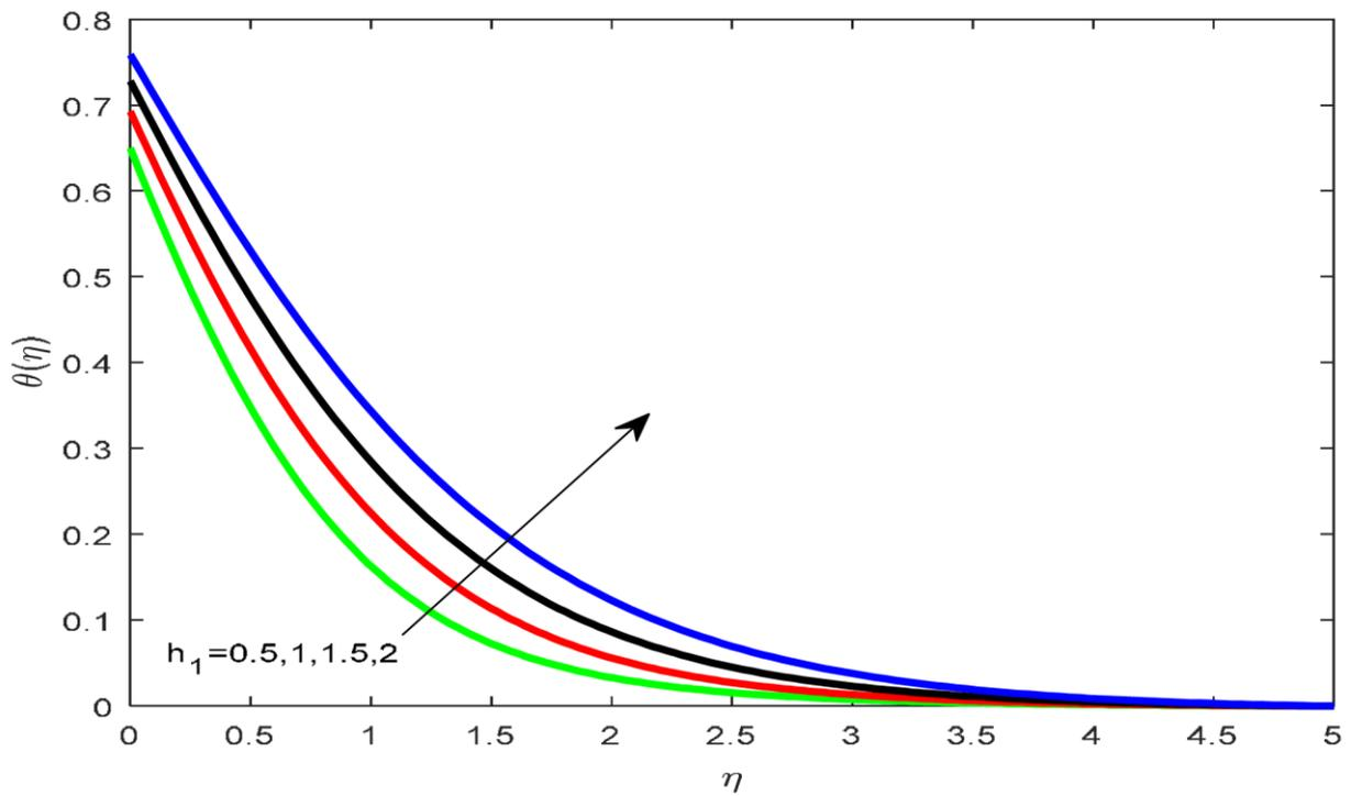
Image.11 Impact pertaining to  $h_I$  based upon thermal field.
