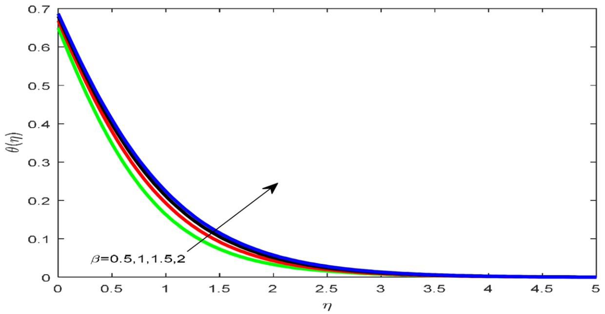
Image.5 Impact pertaining to  $\beta$  based upon thermal field.
