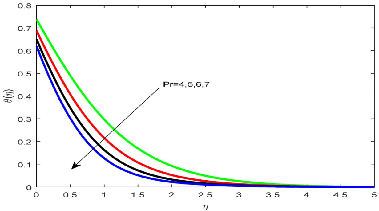
Image.13 Impact pertaining to  $Pr$  based upon thermal field.
