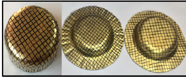
Figure (17): Final blank shapes with different BHF's for (CuZn30 sheets-Al foam core).
