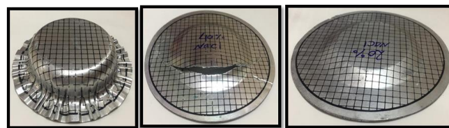
Figure (15): Final blank shapes with different BHF's for (Al1100 sheets-Al foam core).
