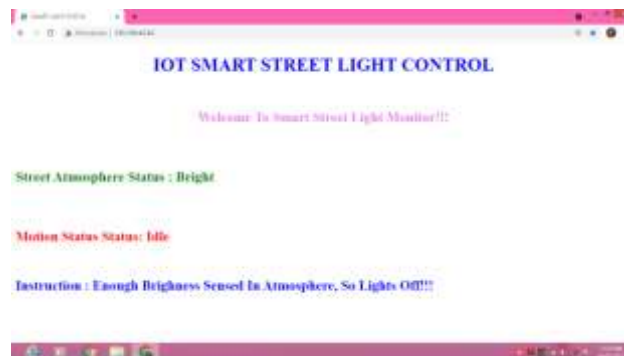
Fig 3.5 LDR detects Brightness (Day Time)
