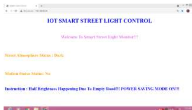
Fig 3.6 LDR detects Darkness (Night Time)
