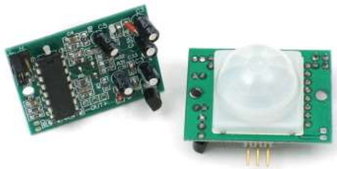
Fig 1.3 PIR - Motion Sensor
