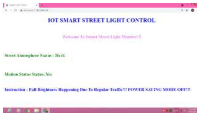
Fig 3.7 LDR and PIR detects Dark and Object movement (Night Time)
