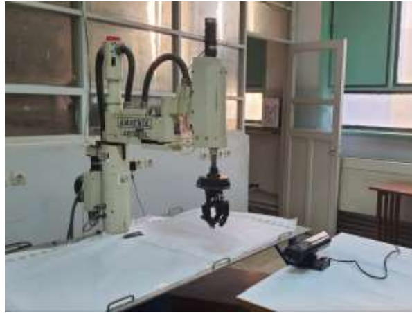
Fig. 5. SCARA robot attached with the three finger under actuated gripper.
