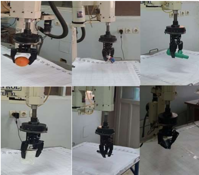
Fig. 11. Stable grasp of six different objects using 3-finger underactuated gripper attached to SCARA robot
