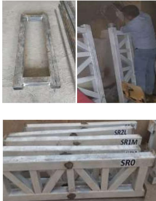
**Figure -3.** Fabrication of specimens and casting.
