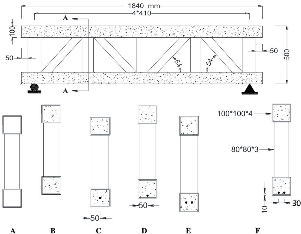
**Figure -2** Specimen details, (A) Hollow specimens ,(B) without any reinforcement (C) reinforced by 1Ø10mm at middle (D) reinforced by 1Ø10mm at lower (E) reinforced by 2Ø10mm at middle (F) reinforced by 2Ø10mm at lower.
