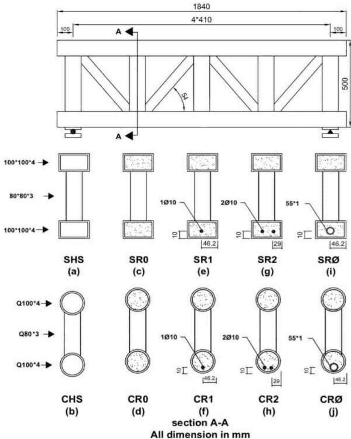
Fig. 2 Detail of specimens
