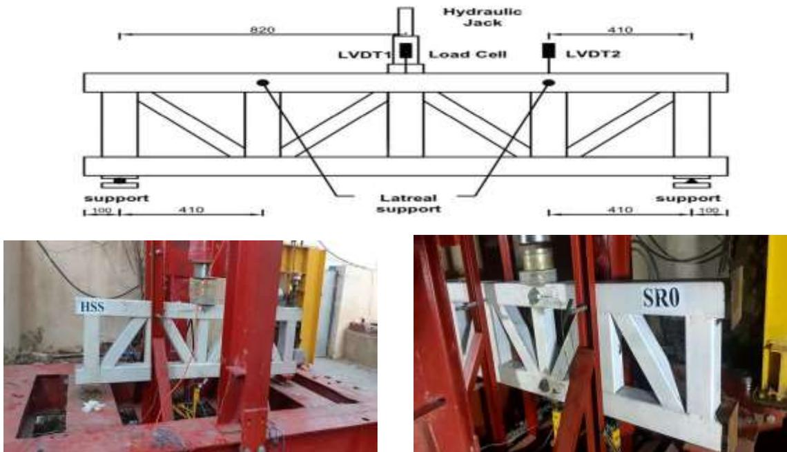
**Fig. 4** Test setup (unit in mm)
