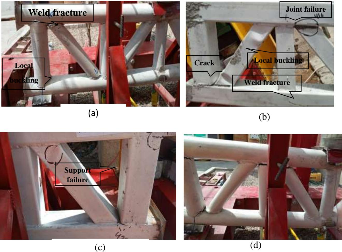
**Fig. 9** Shapes of failure.
