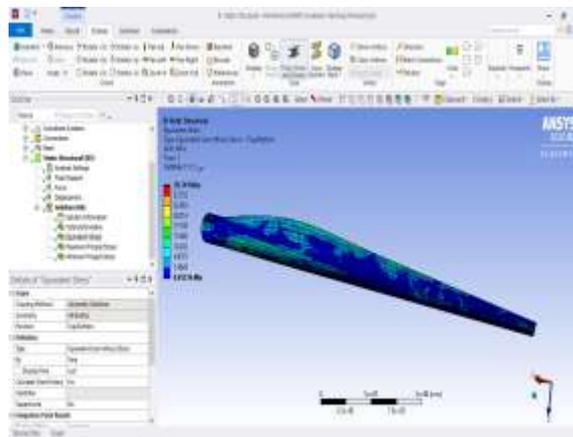
**Figure 10.** Von-Mises Stress Effect
