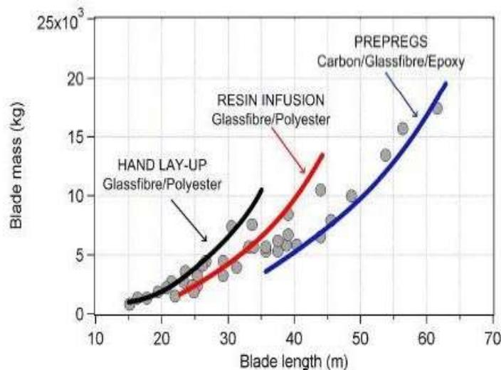
**Figure 5.** Growth of blade mass with blade length
