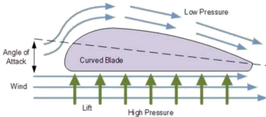
**Figure 4.** Aerodynamic force effect on the blade
