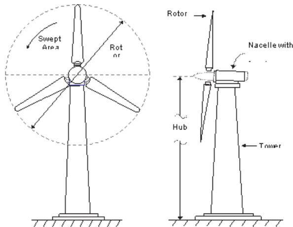
**Figure 6.** Schematic Diagram of Wind Energy System
