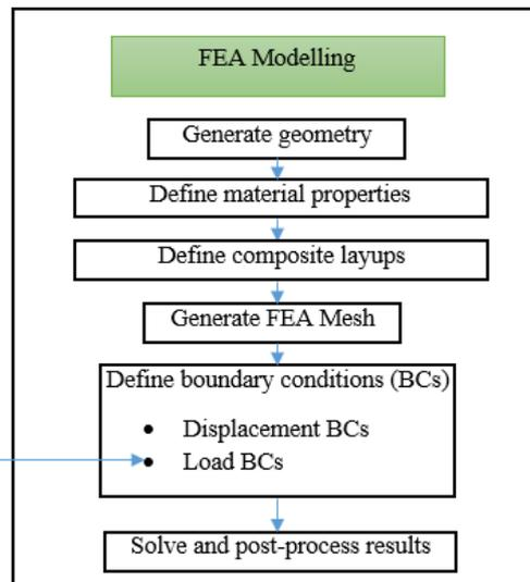
**Figure 7.** Finite Element Steps
