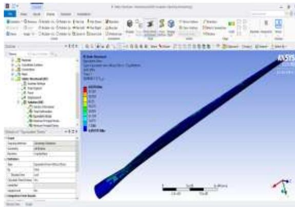
**Figure 12.** Von-Mises Stress Effect on Epoxy Carbon
