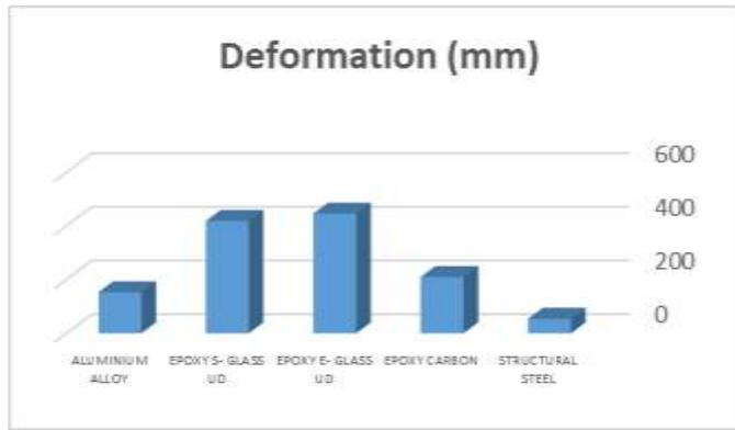
**Figure 20.** Comparison of Deformation of The Blade
