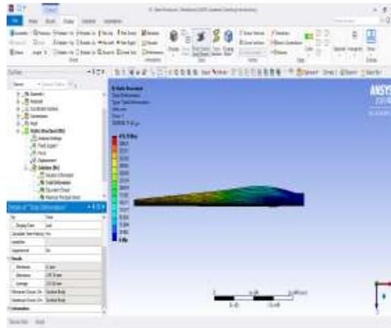
**Figure 15.** Total Deformation Effect on S-glass
