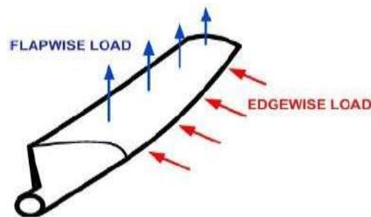
**Figure 3.** Load on wind blade turbine
