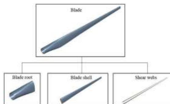
**Figure 1.** Schematic of blade structure
