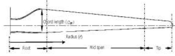
**Figure 2.** A wind blade turbine plan and region classification
