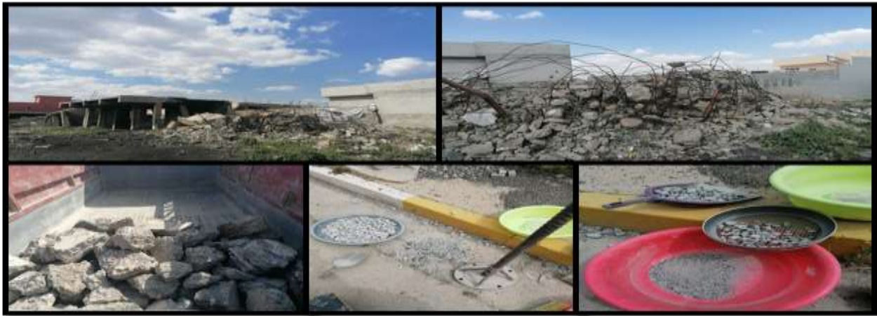
Figure (4) : Concrete rubble and crushed into fine aggregate
