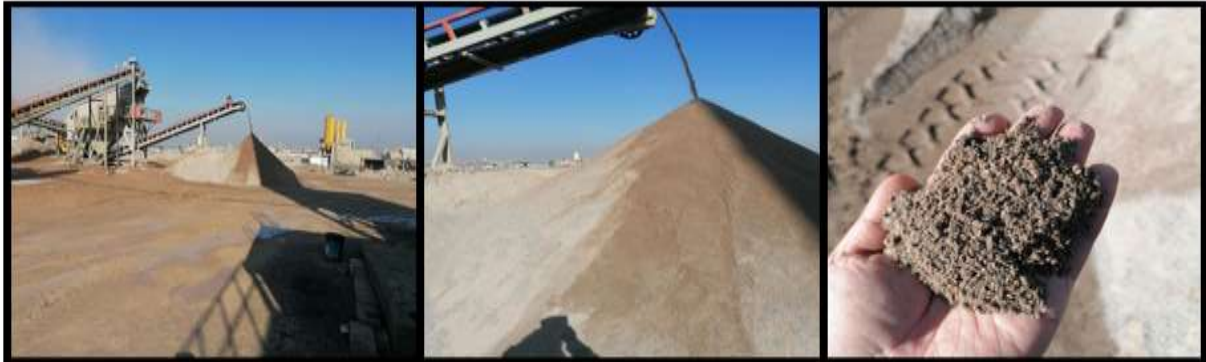
Figure (2) : Fine aggregate (crushed gravel) from the Kukjali blocks and tiles production plant
