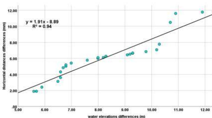
Figure (4.1): Relation model of horizontal distances differences (creep) versus (water elevations head difference) for the period of (2016-2017) within upstream side of the dam
