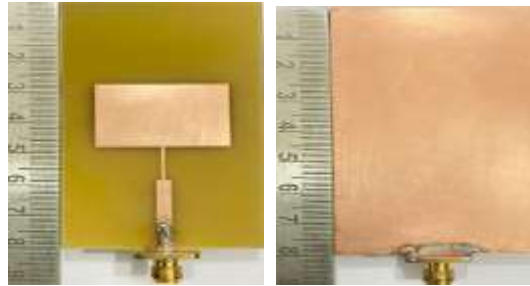
Fig. 2. Fabricated prototype of conventional microstrip antenna.
